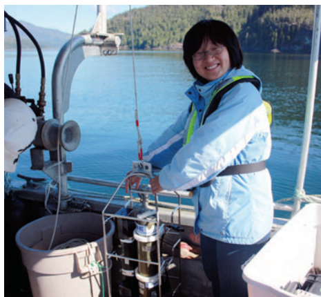
Di Wan with a conductivity, temperature, and depth (CTD) instrument. Photo: Di Wan (UVic)
