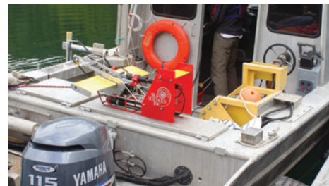
The Acrobat undulating sensor vehicle used in the search for organic particle fish waste plumes. Photo: Stephen Cross (UVic)
