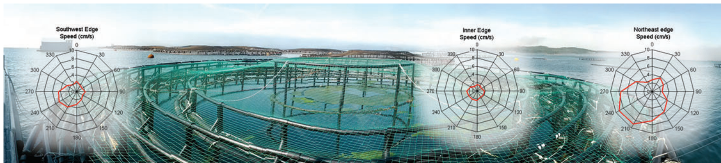
Polar plots of relative current speeds and headings measured at a 5 m depth over several tidal cycles. Plots are shown at their relative locations within a mussel polar circle raft at an IMTA site in the Bay of Fundy. These data help to determine the frequency of particle delivery from Atlantic Salmon cages and how current velocities, around Blue Mussel socks at different locations within the polar circle raft, may affect particle clearance and particle depletion rates of co-cultured shellfish. Photo: Gregor Reid (UNBSJ/DFO – SABS)
