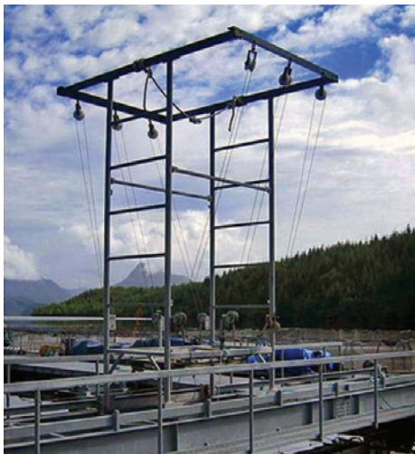
The SEATram shellfish system and hoists developed at the Kyuquot SEAfoods Ltd. IMTA site. Photo: Eric Hovenaars (UVic)
